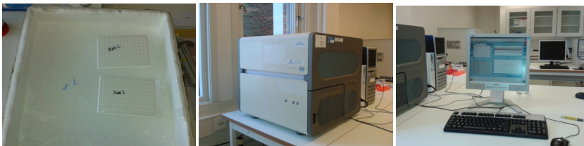
Figure 7: Left – plates ready for adding the primers and SybrGreen-a, middle – Roche™ LightCycler™ 480, right – monitoring the process of amplification on the LightCycler computer program.
