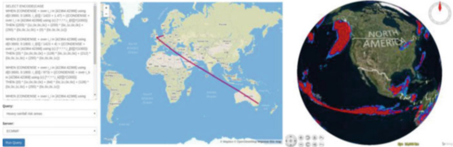
Fig. 16 Visualization of query splitting: original query ( left ), query distribution from Germany to the UK, with subquery spawned to Australia ( center ), query result visualized in NASA WorldWind (Source: EarthServer)
