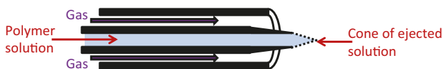
Figure 6.5 The apparatus used for solution blow spinning or melt blowing. (Adapted from Souza, M. A.; Sakamoto, K. Y.; Mattoso, L. H. C. 'Release of the diclofenac sodium by nanofibres of poly(3-hydroxybutyrate-co-3-hydroxyvalerate) obtained from electrospinning and solution blow spinning.' J. Nanomater. 2014 (2014): 129035.)
