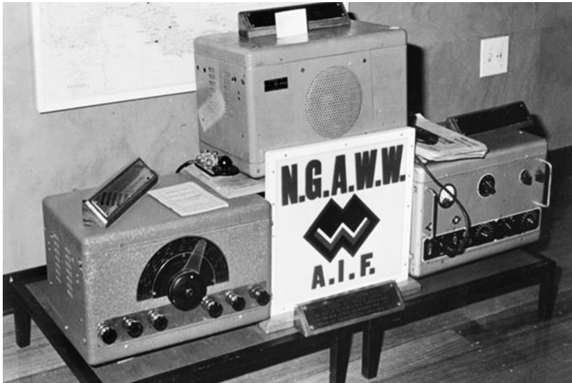
Figure 11: AWA Teleradio 3BZ used by coastwatchers during the war Source: Australian War Memorial (P01035.006).
