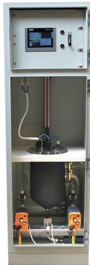
Figure 3.21 Example of a commercial version of a LFS principle-based respirometer using the setup depicted in Figure 3.20. In the middle is the thermostated vessel and at the bottom, left and right, pumps for wastewater and calibration addition (photo: Kelma NV).
