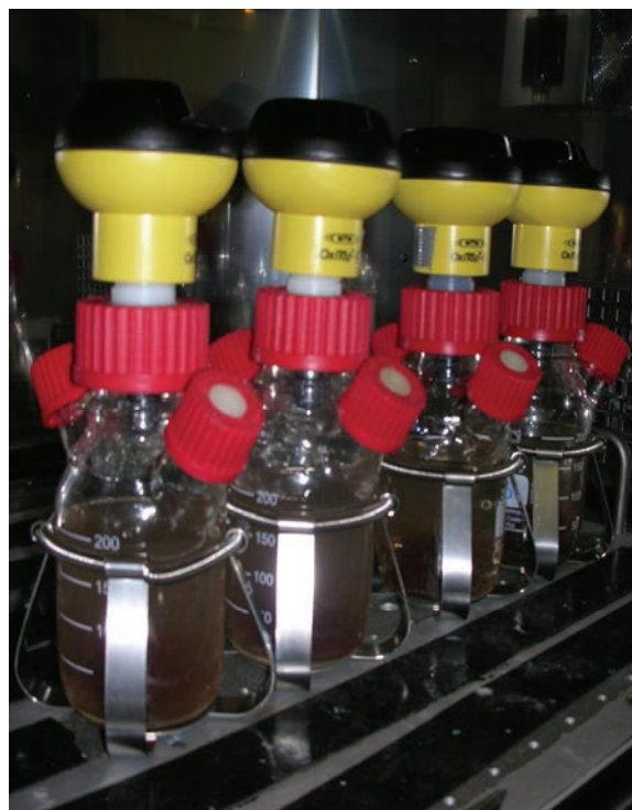
Figure 2.4.2 Commercially available apparatus to perform manometric tests for denitrification purposes (photo: Lotti, 2016).
