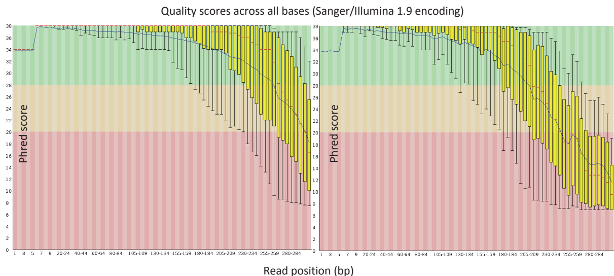
Figure 8.11 Example of Phred quality scores for 2 × 301 bp paired end sequencing of V1-3 16S amplicon libraries on an Illumina MiSeq. To the left is a typical plot for Read1 and to the right is a typical plot for Read2. Read position is plotted versus Phred score. The blue line represents the mean score and the boxplots visualize the score spread. The green area indicates good quality, yellow is reasonable and red is poor. The quality drops towards the end of the read. The quality overview was generated using the FastQC software v0.11.3.
