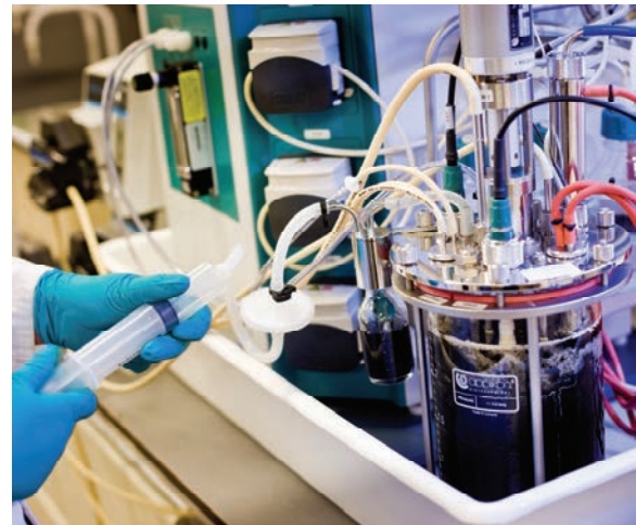
Figure 2.3.11 Collection of a liquid sample to determine the activity of sulphate-reducing bacteria (SRB). Note the characteristic black colour of the enriched SRB biomass in the reactor (photo: KWR Waterycle Research Institute, 2014).
