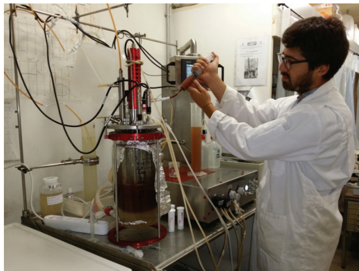
Figure 2.4.15 Execution of batch activity tests. Note the characteristic reddish colour of the enriched anammox culture (photo: Lotti, 2015).
