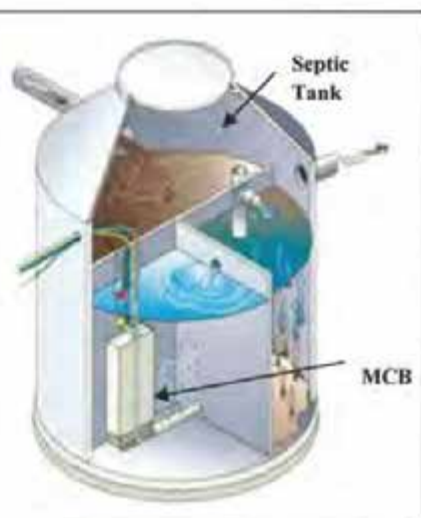
Figure 13: MBR Septic Tank
