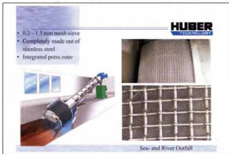
Figure 2: Preliminary Treatment by Rotating Fine Screens
