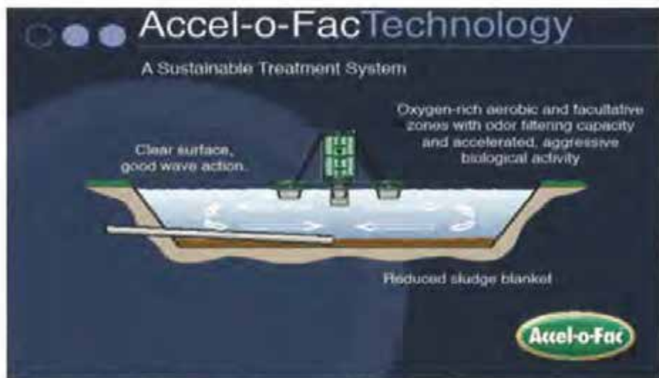
Figure 12: The Mechanism of Improvement in Facultative Lagoons Performance by the use of LAS Mixers, Courtesy LAS International
