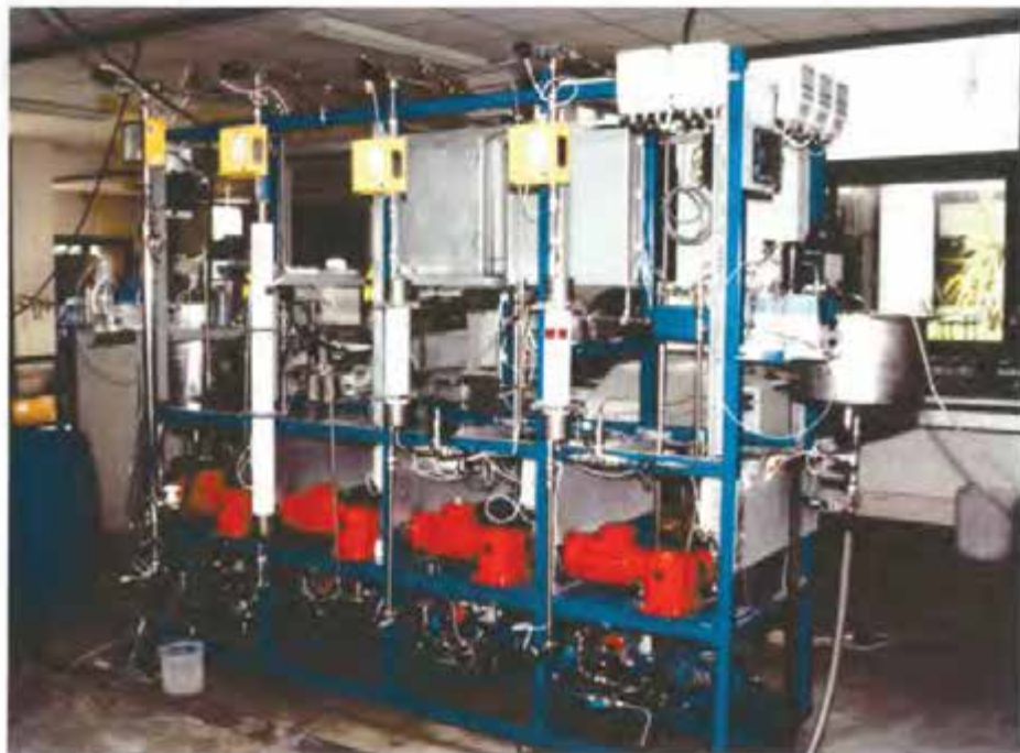
Figure 1: The Grey Water Treatment Unit
