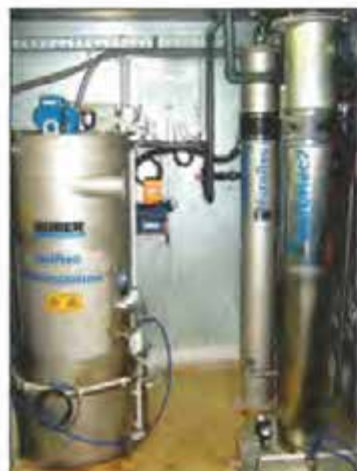
Figure 3: Photo and operational data of our NuRec system with MAP precipitation reactor, stripping and absorption columns
