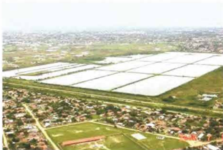
Figure 9: Air Photo of a Conventional Anaerobic-Facultative Lagoons Wastewater Treatment Plant in the City of Santa Cruz, Bolivia
