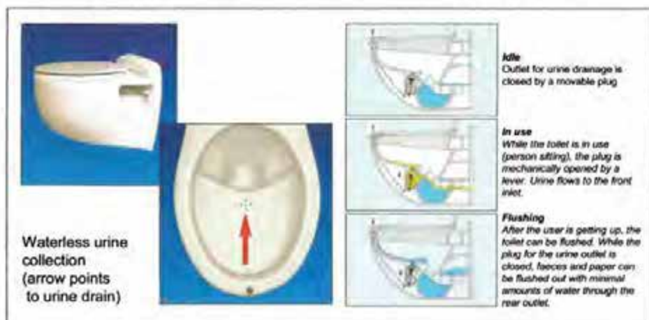
Figure 2: Gravity separation toilet (No Mix-Toilet) of the company Roediger
