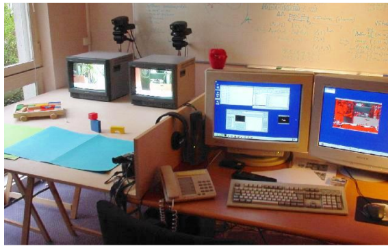
Figure 10.7: The installation for the case grammar experiments used a more sophisticated vision system and objects that could be moved around. We see the two Talking Heads cameras in the background. They are oriented towards objects on the table or situations in the environment. The monitors show the camera images and the states of image processing, just as for the original Talking Heads experiment.
