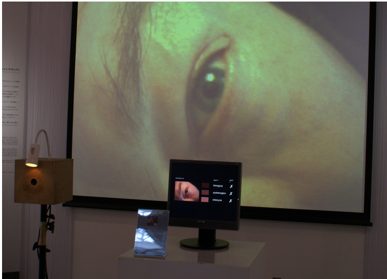
Figure 9.12: Installation at the Tokyo Explorascience Museum. The box is in the left corner. The eye is projected on a big screen. A smaller screen shows the image captured by the camera, the colours recognised, and the words used by the agents.
