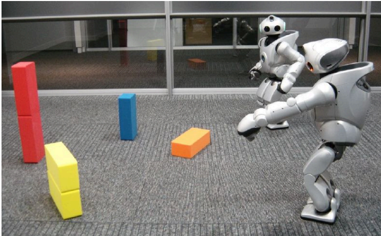
Figure 11.1: Set-up for the Grounded Proper Naming Game. Two Qrio robots are playing a game of reference about individual objects in their environment. They are using proper names and hence have to recognise objects as individuals.
