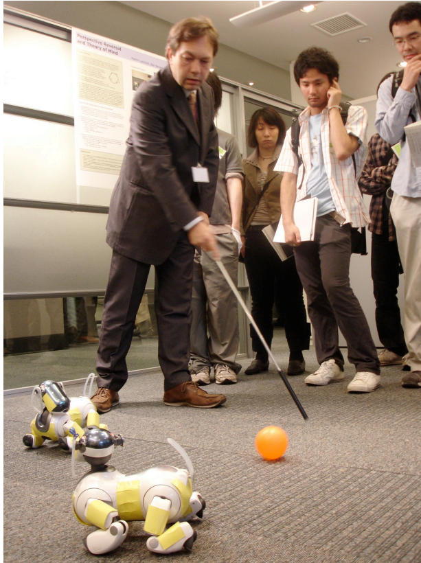
Figure 10.3: Luc Steels demonstrates live the Perspective Reversal experiment in Tokyo, April 2005. AIBO robots track the movement of a ball and the robot acting as speaker describes to the hearer an observed movement, possibly taking into account the perspective of the hearer. For example, the speaker might say the ball rolls from my left to your right .
