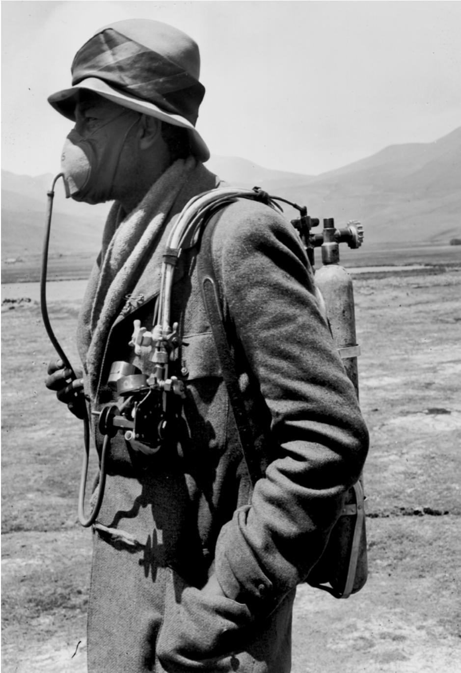
Image 2.2. The oxygen apparatus, invented by George Finch, used on the 1922 and subsequent Everest expeditions.
