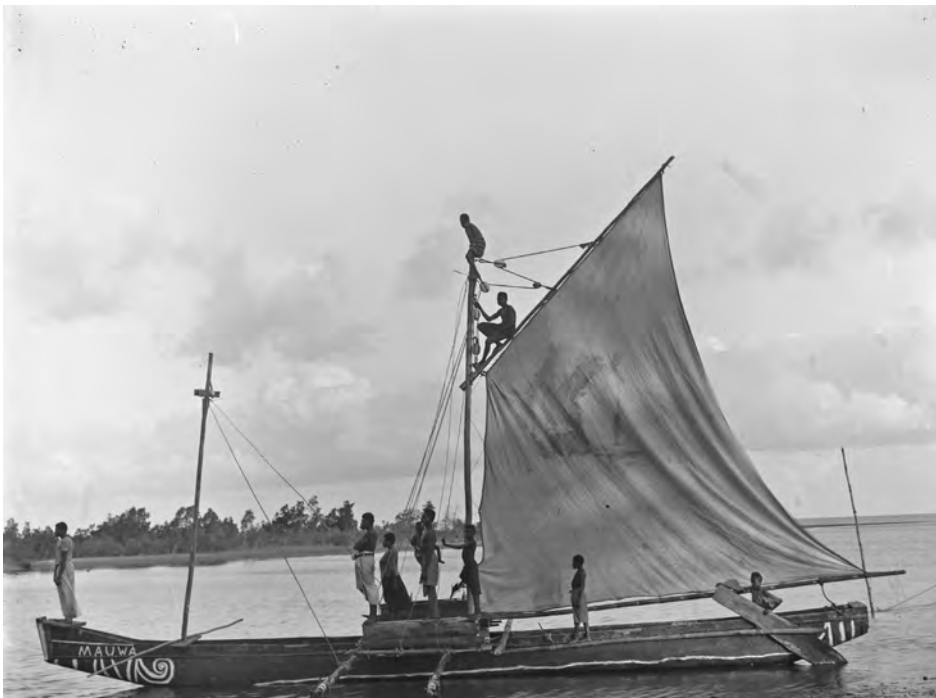
Figure 28. The motomoto , Mauwa , being prepared for sail at the mouth of the Binaturi River (VKK 248: 431). At that time canoes were only fitted with half-platforms and small standing areas on the bow and stern. Later on the large ocean going canoes were fitted with full platforms and the inside of the canoe was used for storage and equipment
