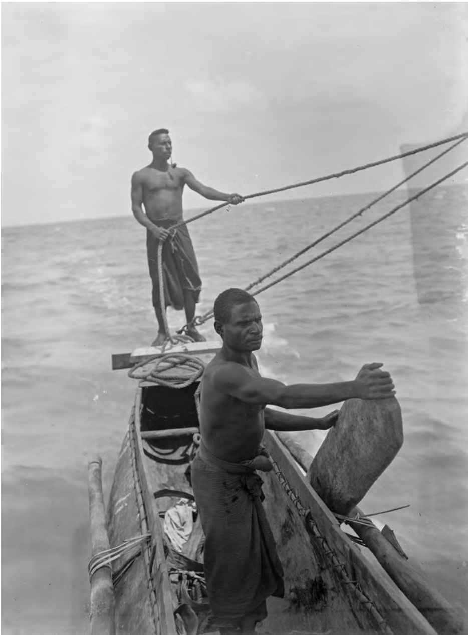
Figure 29. Photograph illustrating the method of steering using a movable steering board placed on the lee side of the canoe (VKK 248: 436)
