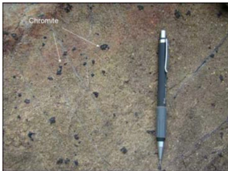
Fig. 2: disseminated chromite grains (black) in La Cabaña serpentinite. Nickeline Irsite Os alloy Chromite Laurite Millerite Irsite
