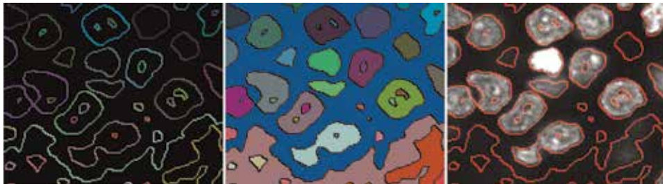
Figure 4. Connected components of the Laplacian operator's zero space. The boundary (left) is overlaid on the cell nuclei image (right). The connected components (center) are calculated from Laplacian of Gaussian, s = 12 .
