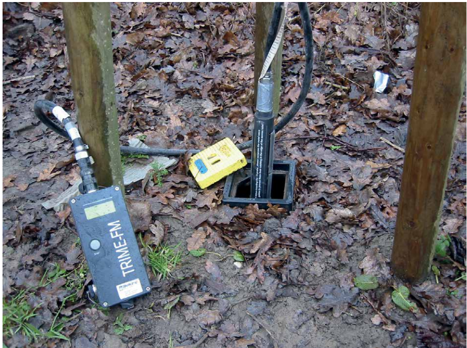
Figure 4. Groundwater level, flow and chemical composition, especially the oxygen content, determine the preservation potential of invisible heritage within the subsurface. Groundwater monitoring is needed to identify changes in hydrological parameters, caused by e.g. construction and the potential impacts of reduced groundwater on the conservation of archaeological deposits.
