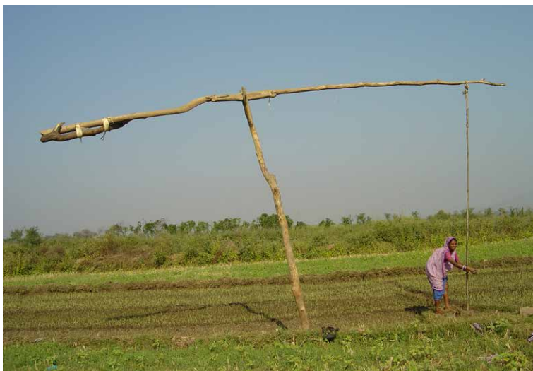
Figure 2. Traditional Water Lifting Device, Orissa. Photograph: Ganesh Pangare.
