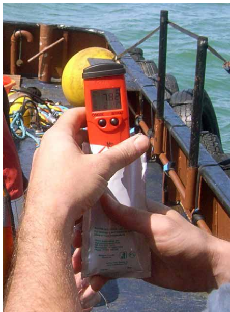
Figure 3. Archaeologists commencing the first systematic programme of bed-level pH baseline recording in the UK. The use of such data will, in the long term, assist in the management of change (Wessex Archaeology for English Heritage).
