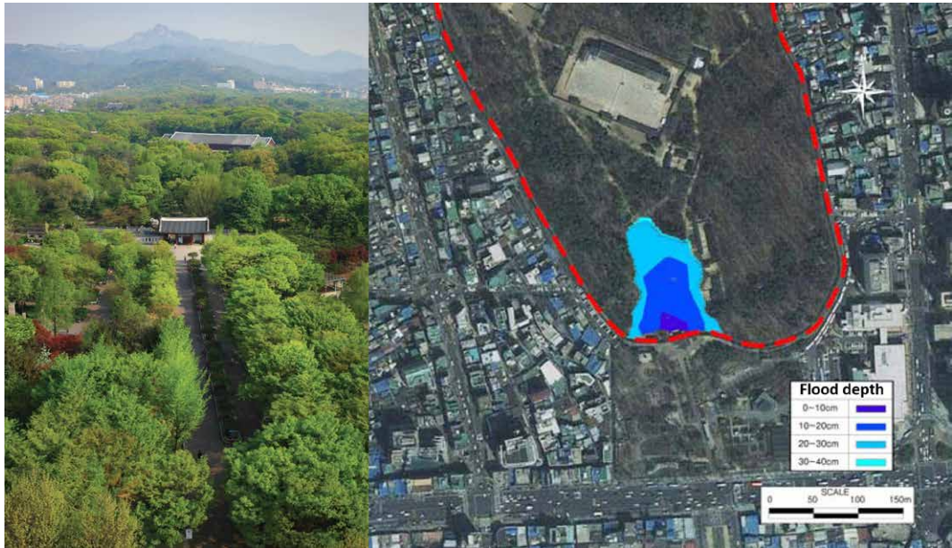
Figure 5. Jongmyo Shrine near the central business districts of Seoul and the flood inundation map of the 180-minute duration rainfall with a 200-year return period (Cultural Heritage Administration of Korea; NRICH 2012).
