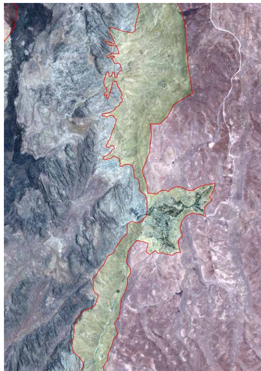
Figure 3. Geologic zones pertinent to Petra hydrology. Limestone highland formation to the right, sandstone formation in which Petra is located to the left, unconformity and spring zone in the center.
