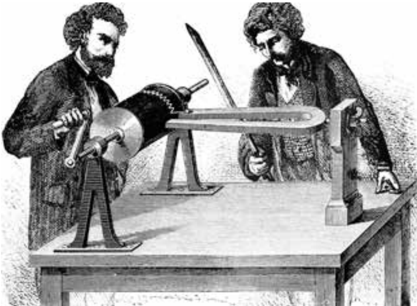
Figure 3.1 Graphical method of observing the mode of vibration of a tuning fork (Lockyer 1878, 167). The tuning fork seems to be too large to be brought in vibration by the small bow. This picture is probably meant for explaining the principle and not a realistic picture of how the experiment was executed.
