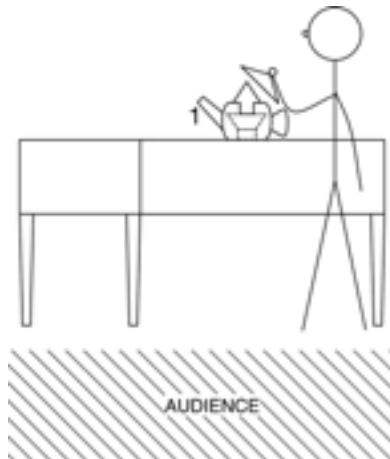
Scheme 5.1 Alvin Lucier Nothing Is Real (Strawberry Fields Forever) : a small loudspeaker is put in a teapot. By moving the teapot lid the sound radiated by the small loudspeaker is modified.
