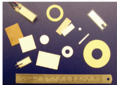
Figure 3. PZT and PVDF of various sizes and shapes [14]
