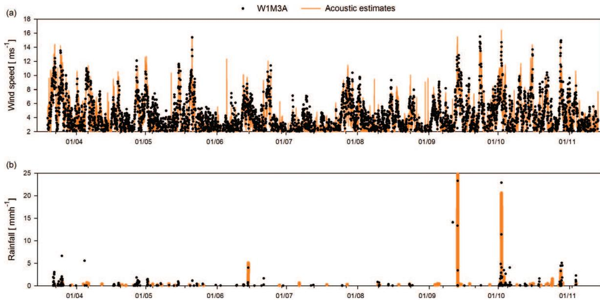
**Figure 6.** Time series of (a) wind speed and (b) rainfall as measured by the anemometer and the rain-gauge installed on the W1M3A marine observatory, and the estimates obtained from acoustic samples.
