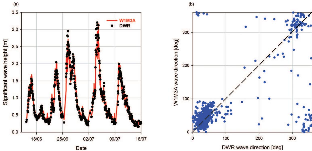
**Figure 2.** (a) Time series of significant wave height as estimated through the acoustic wave meter system and measured by the Datawell Waverider buoy. (b) Scatter plot of the wave direction estimated by the acoustic wave meter versus the one measured by the Datawell Waverider buoy.
