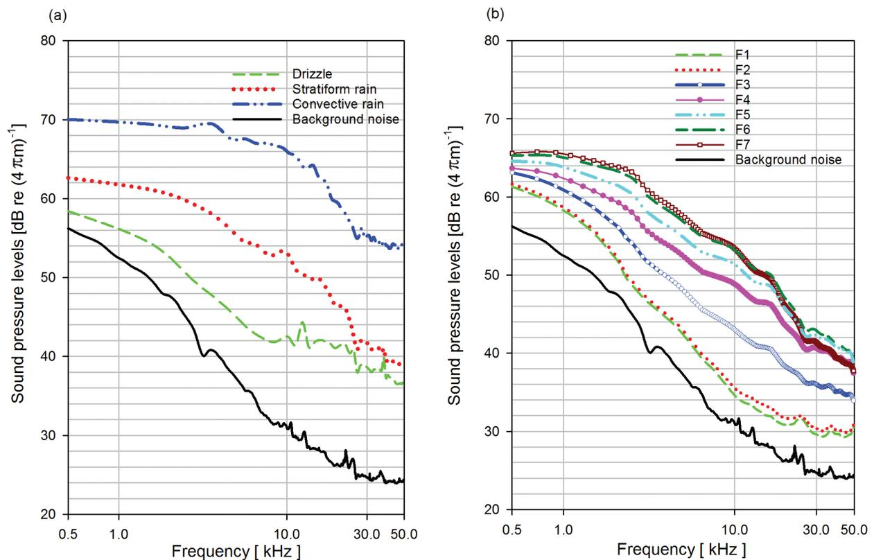
**Figure 5.** Average sound spectra for (a) different types of precipitation and (b) wind speed greater than 2 ms<sup>-1</sup> subdivided in Beaufort classes compared to the average spectrum of the background noise.
