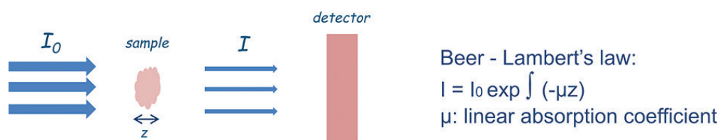
Figure 1. Optical absorption and the Beer-Lambert's law.
