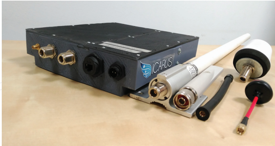
Figure 4. SUGV COM box and set of antennas used in various missions. (Source: ICARUS).
