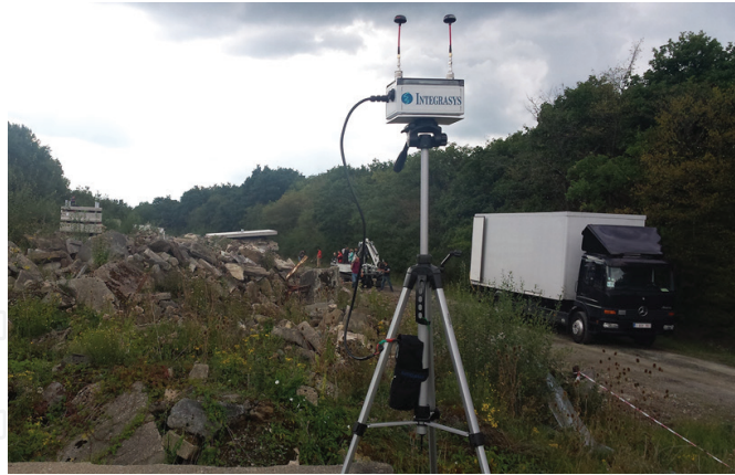
Figure 9. ICARUS COM tools communicating to rescue workers operating inside a rubble field. (Source: ICARUS).
