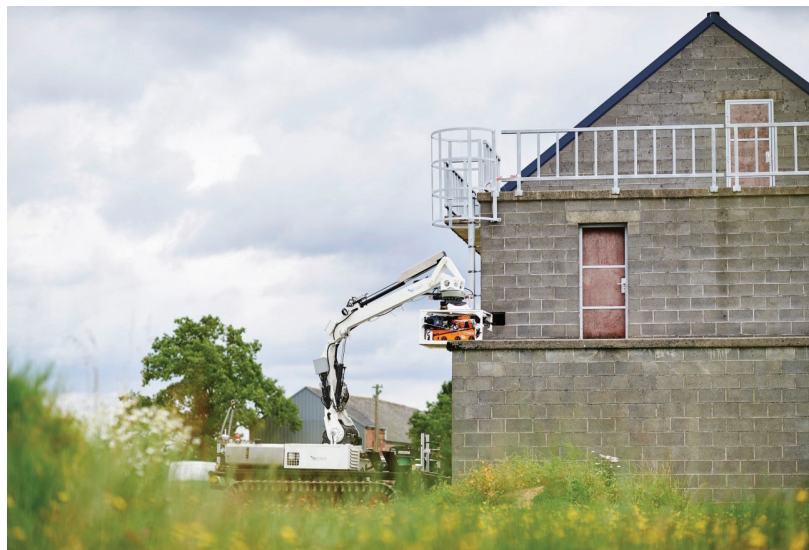
Figure 12. ICARUS large unmanned ground vehicle deploying the small unmanned ground vehicle on the top of a building (source: ICARUS).
