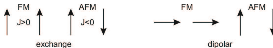
Figure 1. Exchange vs. dipolar interactions. Preferred configuration of magnetic moments depends on the sign of the exchange integral J for the exchange interaction while on the alignment of magnetic moments for the dipolar interaction.
