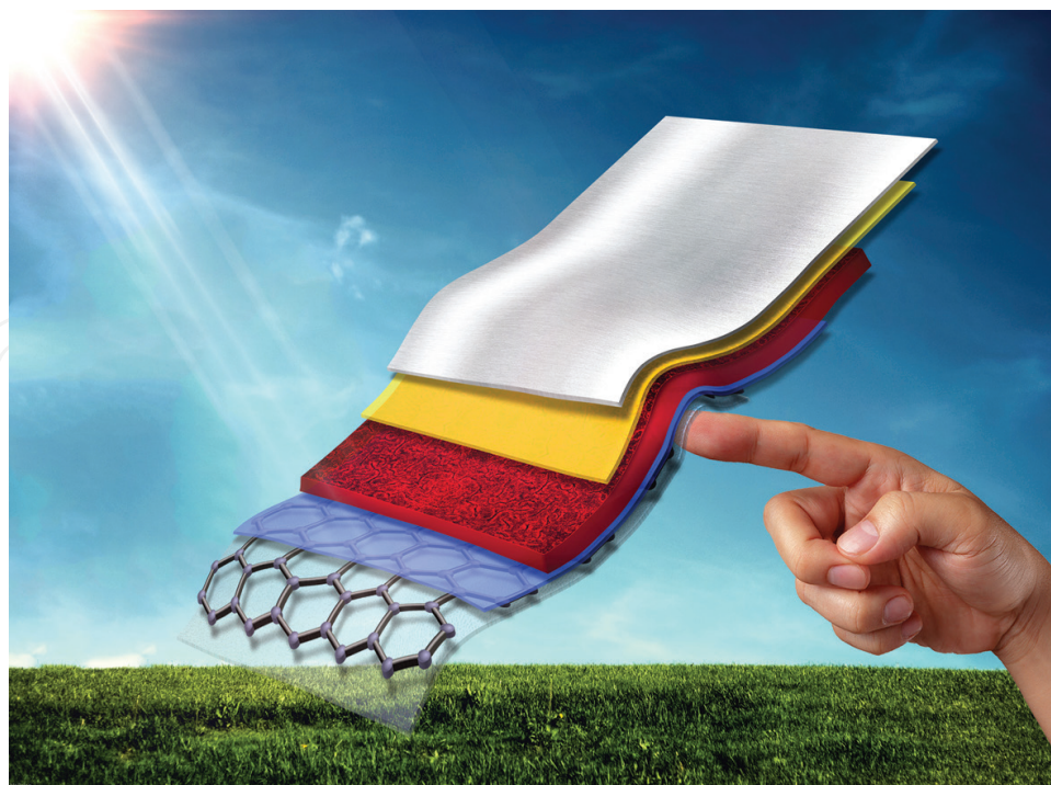
Figure 1. The graphene-based TCE as the anode in a typical flexible OSC.
