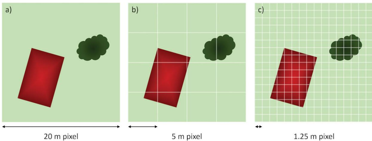
**Figure 3.** Relationship between objects under consideration and spatial resolution in urban sites: (a) pixels significantly larger than objects, (b) pixel and objects sizes are of the same order, and (c) pixels are significantly smaller than object.
