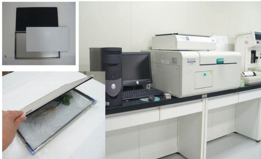
Fig. 4.1 RI (radioisotope) imaging system using an IP. A plant sample containing RI is placed on an IP shown as a white board, and the IP was exposed to radiation from the sample for a time period in a cassette. Then, the radiation image is scanned by a scanner, and the RI amount is analyzed by a computer
