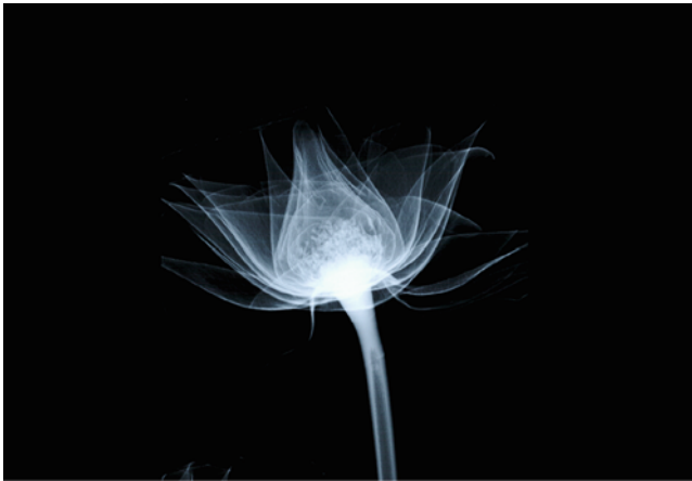
Fig. 1.19 Water image of a rose flower by the neutron beam
