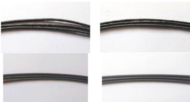
Fig. 10.30 Extrusion trials of HDPE based filament at different screw rotational speeds and temperatures
