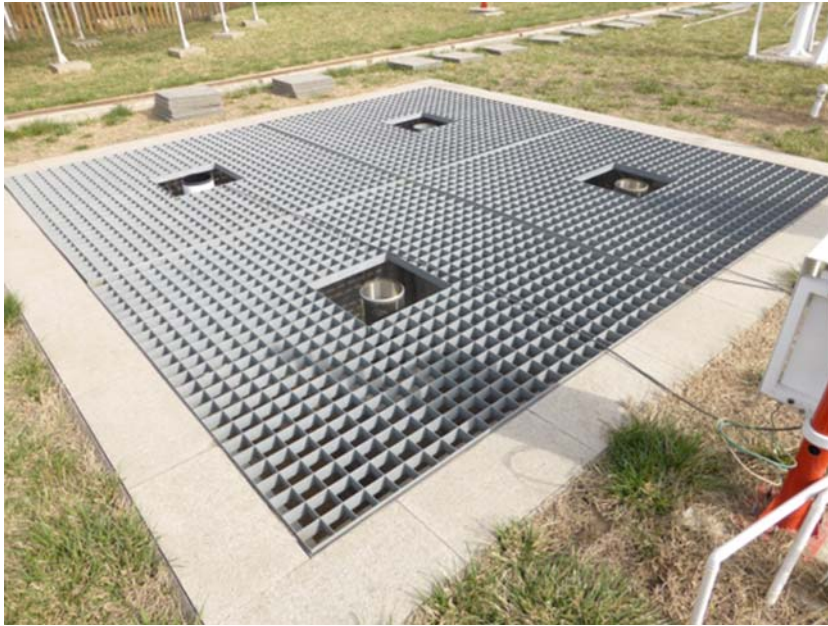
Figure 2.3 Pit rain gauges or collectors. Source: Thomas Einfalt (hydro & meteo GmbH).
