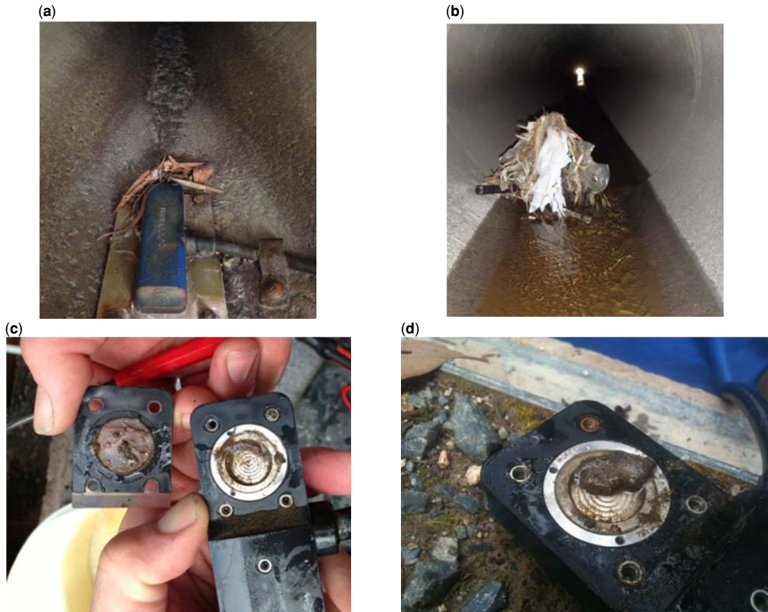
Figure 4.3 Debris caught on sensors blocking sensor beams (a, b), sediment on diaphragm of a pressure sensor (c, d). Source: Peter Poelsma, University of Melbourne.
