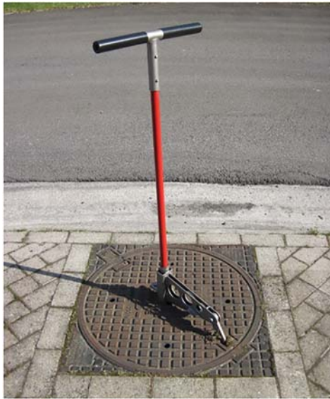
Figure 7.3 Ergonomic lifter for manhole covers developed by Aquafin NV. Source: courtesy of Jan Swankaert (Aquafin NV).
