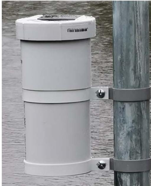
Figure 7.16 Self-powered water level monitoring system using three AA rechargeable batteries and a 0.5 W solar panel (on top). The data are sent every 15 minutes using the SigFox network – wetland in Melbourne, Australia. Source: Frédéric Cherqui (INSA Lyon).
