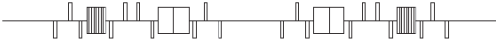
Figure 4.19: A basic QBA cell. Several QBA cells can be grouped together to form a superperiod with different optical properties in the straight sections.
