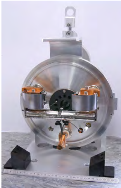
Fig. 2. The interior of a target unit showing the suspended tantalum oven containing the target material.
