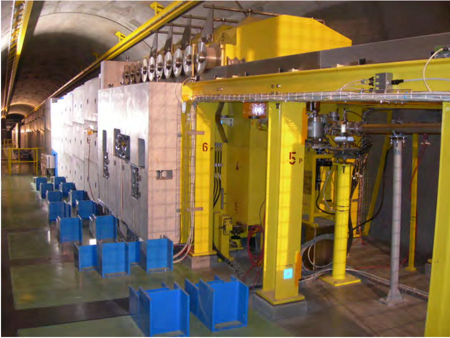
Fig. 9. Photo of the CNGS target cavern with the target station in the forefront. The slope of the tunnel required to point to Grand Sasso is visible.
