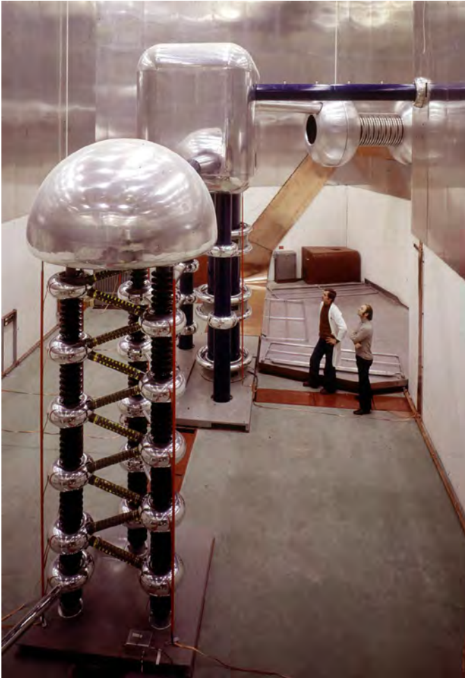
Fig. 4. The Cockcroft–Walton-type accelerator for the CERN LINAC2 linear proton accelerator generated a voltage of 750 kV and was used up to the late seventies [13].
