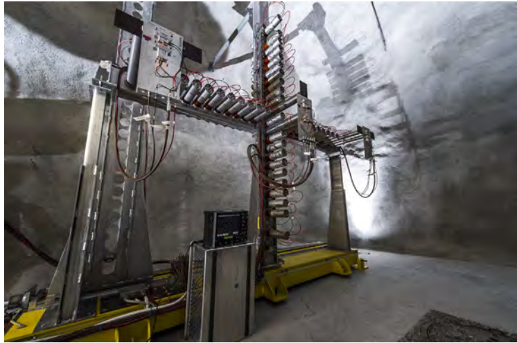
Fig. 13. Right: An LHC ionization chamber (BLM monitor) used for the CNGS muon station. Left: The muon monitoring station equipped with 42 ionization chambers.
