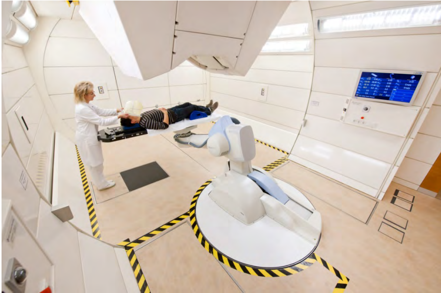
Fig. 4. Patient positioning procedure at the HIT gantry treatment place — for rotation of the gantry the closed folding ground floor is bent down.
