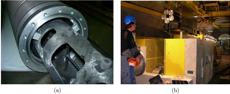
Fig. 6. The CNGS target. (a) Detail of a target head with the graphite rods, the support structure and the external aluminium cylinder, (b) photo during the installation of the target unit with the five heads in its place in the beam. The side iron and marble shielding and the forced-air duct at the bottom are visible. In the final installation a top shielding with remotely movable blocks is installed.
