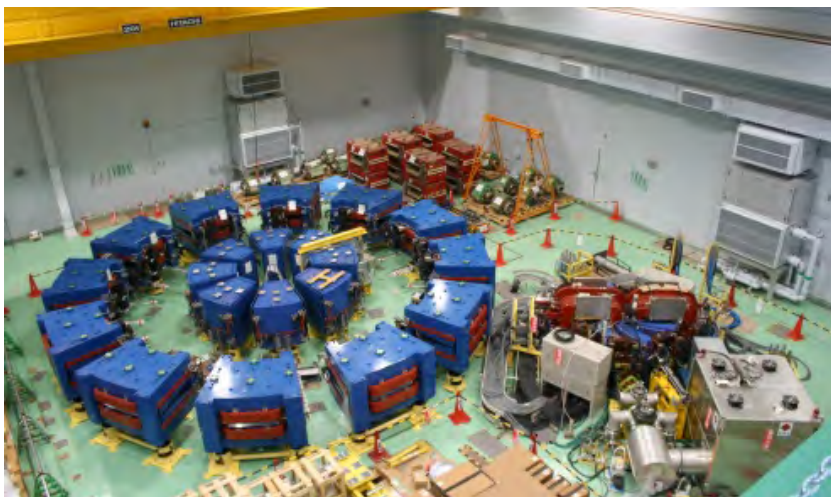
Fig. 6. FFAG complex at KURRI for ADSR experiment [Aiba (2000); Mori (1999); Pyeon (2009)].
