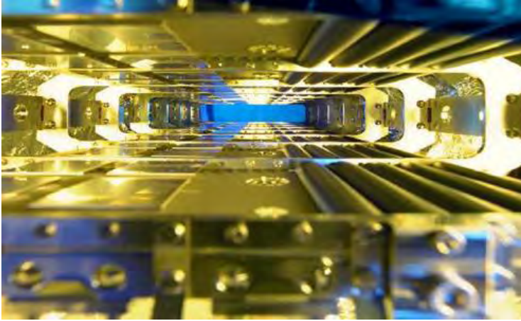
Fig. 10. View through the aperture of stochastic cooling pick-ups installed in the gap of the dipole magnet in the center of the northern arc of the ESR, where the dispersion amplitude has a maximum value of 6.3 m. The correction electrodes are installed in the center of the southern arc. The hot beam on the injection orbit (left side) is passing through the electrodes where it can be pre-cooled before it is decelerated by means of RF to the permanently electron-cooled stack (right side) for beam accumulation (RF-stacking). For mass measurements, electron cooling is applied at injection energy immediately after stochastic pre-cooling (see Fig. 11).
