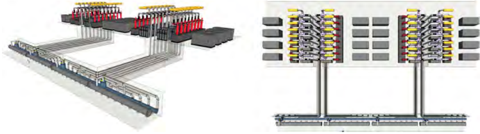
Fig. 2. The ESS RF sources in and the RF waveguide stub lay-out. The 3D view on left and the view from top on right.
