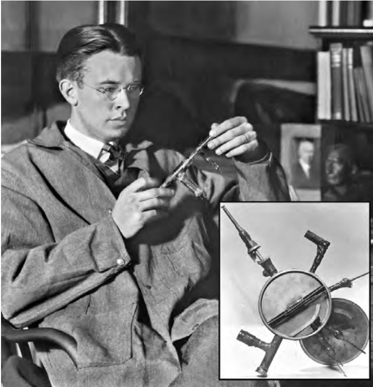
Fig. 13. Ernest Lawrence with the first 5 inch Cyclotron. The device accelerated H^- ions to 80 keV but was compact enough to fit easily into a hand [23].
