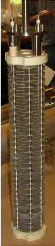
Fig. 13. Right: An LHC ionization chamber (BLM monitor) used for the CNGS muon station. Left: The muon monitoring station equipped with 42 ionization chambers.
