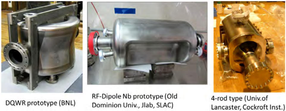
Fig. 16. The three types of compact crab cavities that are being pursued at the moment for the HL-LHC.
