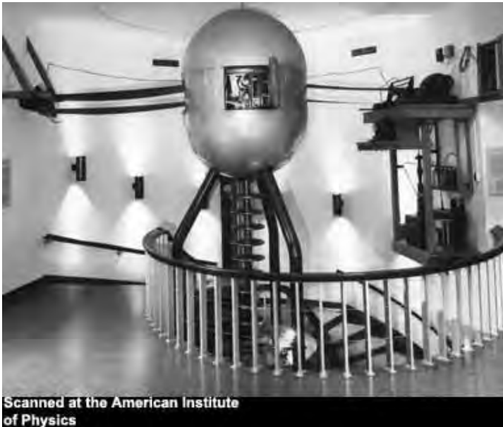
Fig. 6. The Million Volt Van de Graaff voltage terminal used by Tuvé for proton-proton scattering experiments in 1931 [17].
