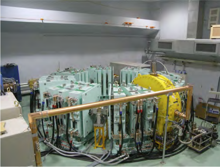
Fig. 9. FFAG-ERIT for intense neutron production.
