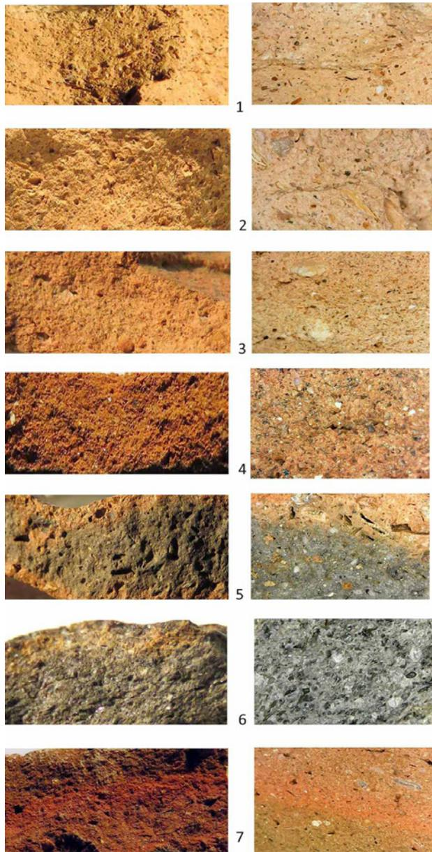
Figure 9.4. Fresh fractures of samples 1-7, left macro, right digital microscope, 100x.<sup>5</sup>
