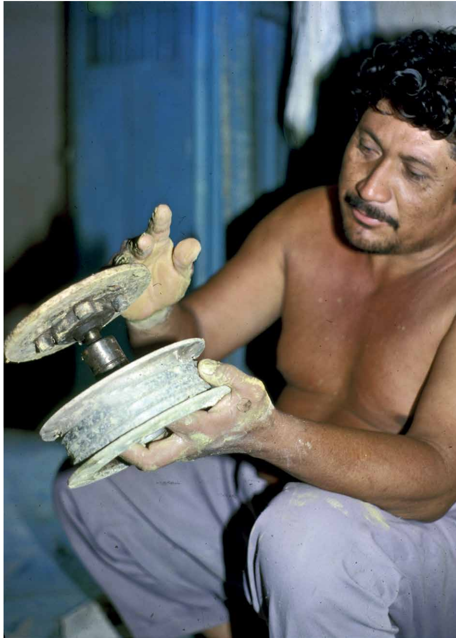
Figure 4. Detail view of the ball bearing turntable created and welded together by a mechanic.
