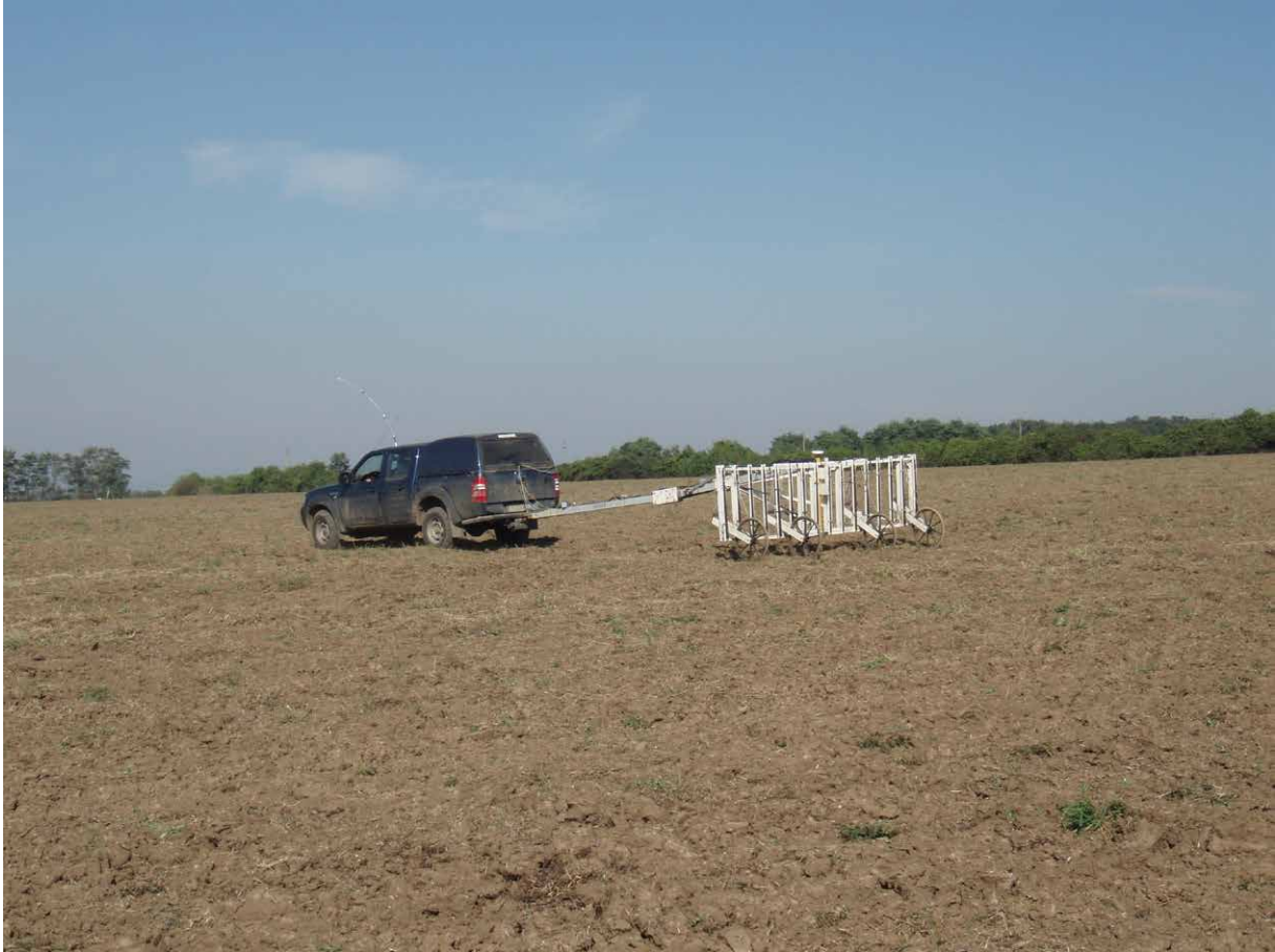
Figure 2.1.4. The 16-channel Magnetometer (SENSYS MAGNETO®-MX ARCH) during a survey in 2008 (photo: K. Rassmann).
