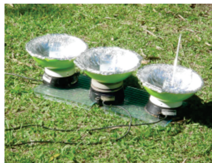
FIGURE 6 – PHOTO OF PHOTOCHEMICAL REACTOR OPERATED WITH SOLAR RADIATION
