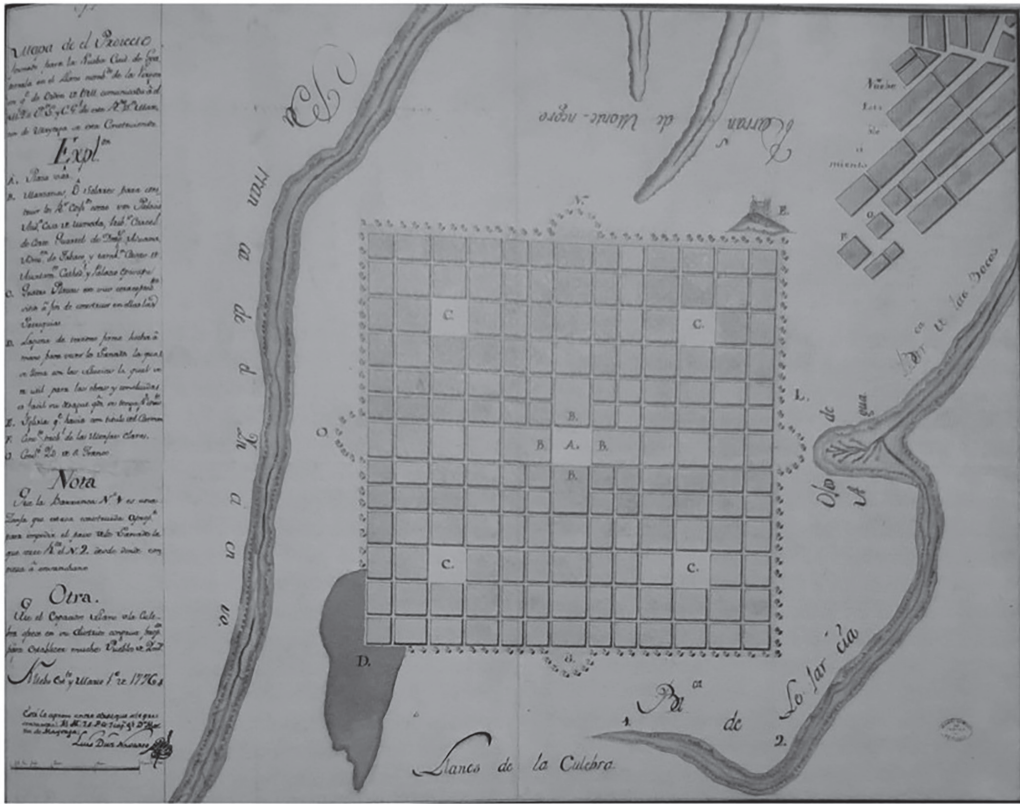
Figure 16.6. Guatemala was then rebuilt on the grid after an earthquake in 1773. Plan of Guatemala, 1776, by Luiz Diez de Navarro. The streets were laid out north-south, east-west (see Sambricio, Territorio y ciudad and Markman, ‘The plaza mayor’).
