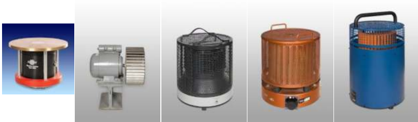
Figure 3.1: Primary and transfer sources used in this study. Left to right: primary source, AEG Type ADEB71K2, Brüel & Kjær Type 4204, EDF Type A and Norsonic Type Nor 278.
