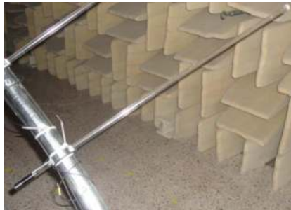
Figure 3.3: Microphone positioned on the scanning apparatus.
