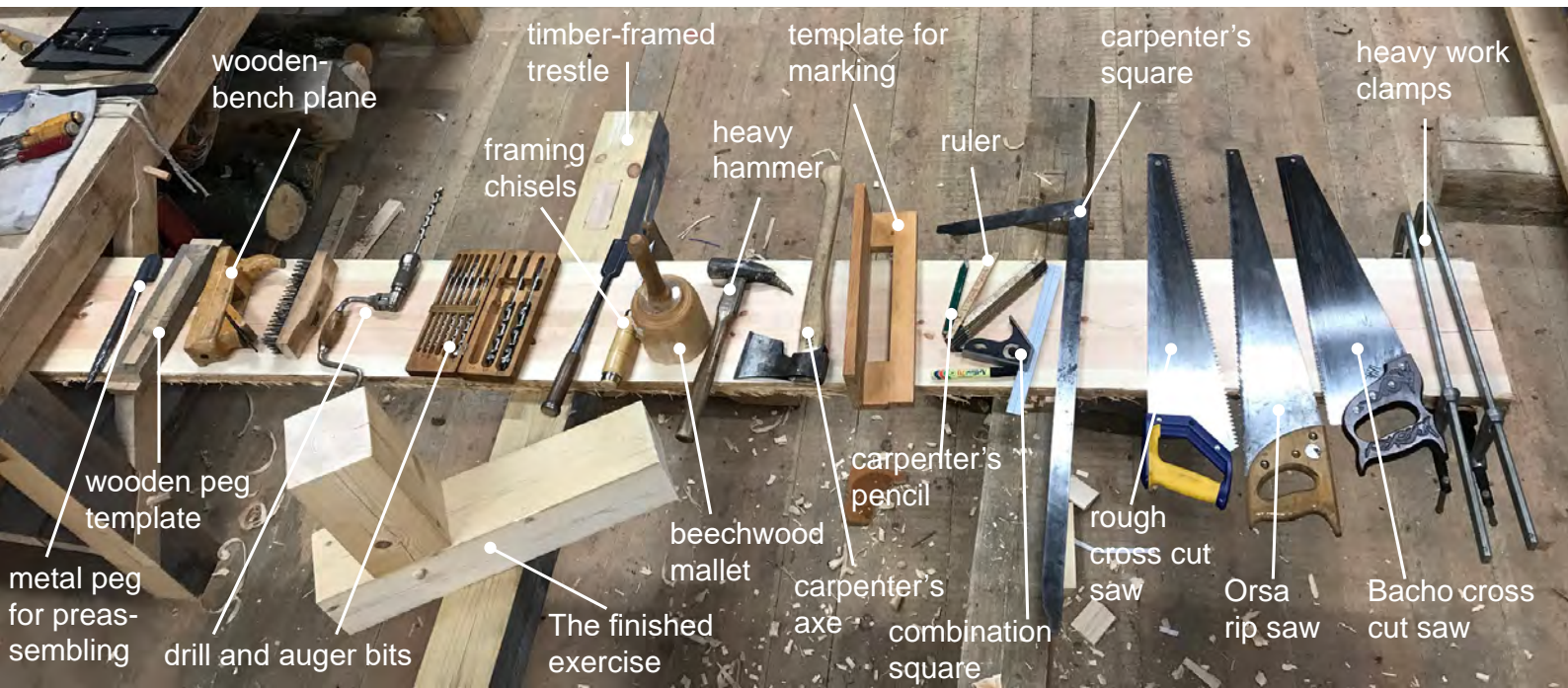
Figure 10: The tools used for the video-based learning resource with the finished exercise in front. Photograph by Ulrik Hjort Lassen.
