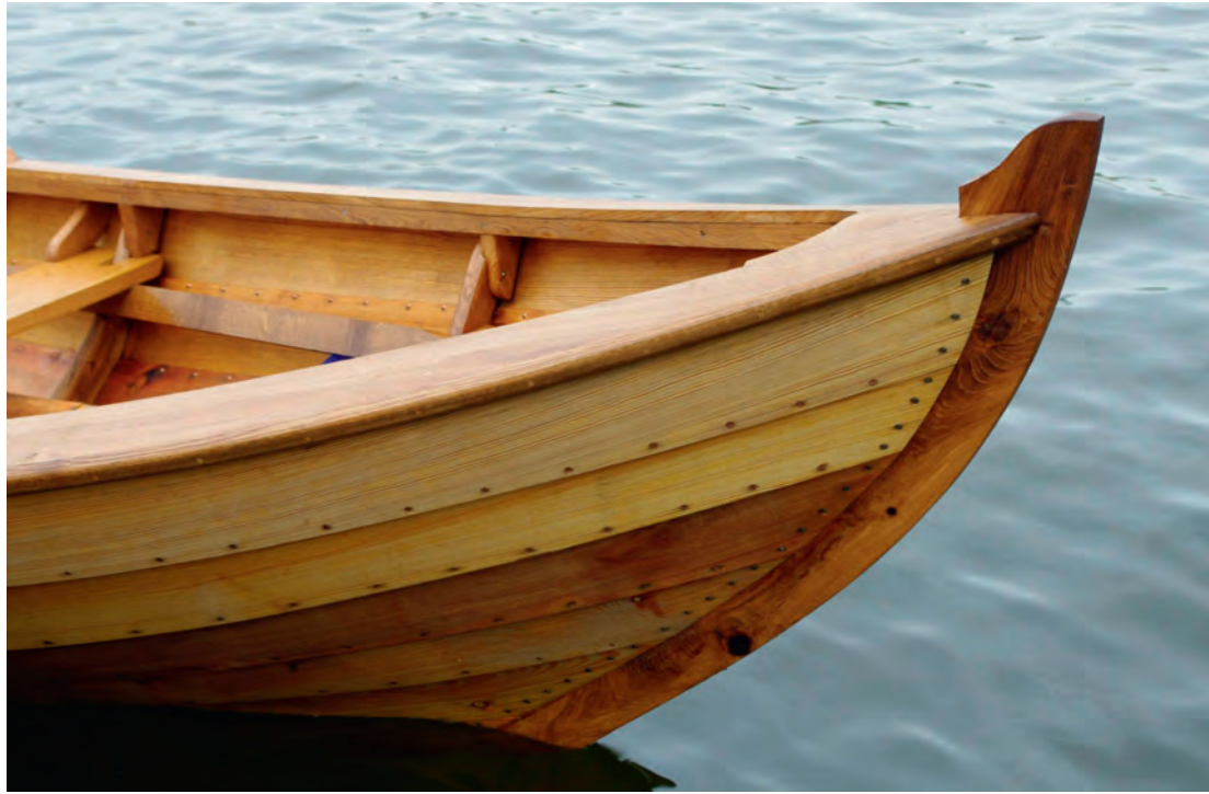
Figure 1: A clinker-built boat, where the planks overlap and are riveted together with copper rivets. Local types of wood are used, and the boat builder will hand-pick grown bends and high-quality wood. Photograph by Rikard Plog.
