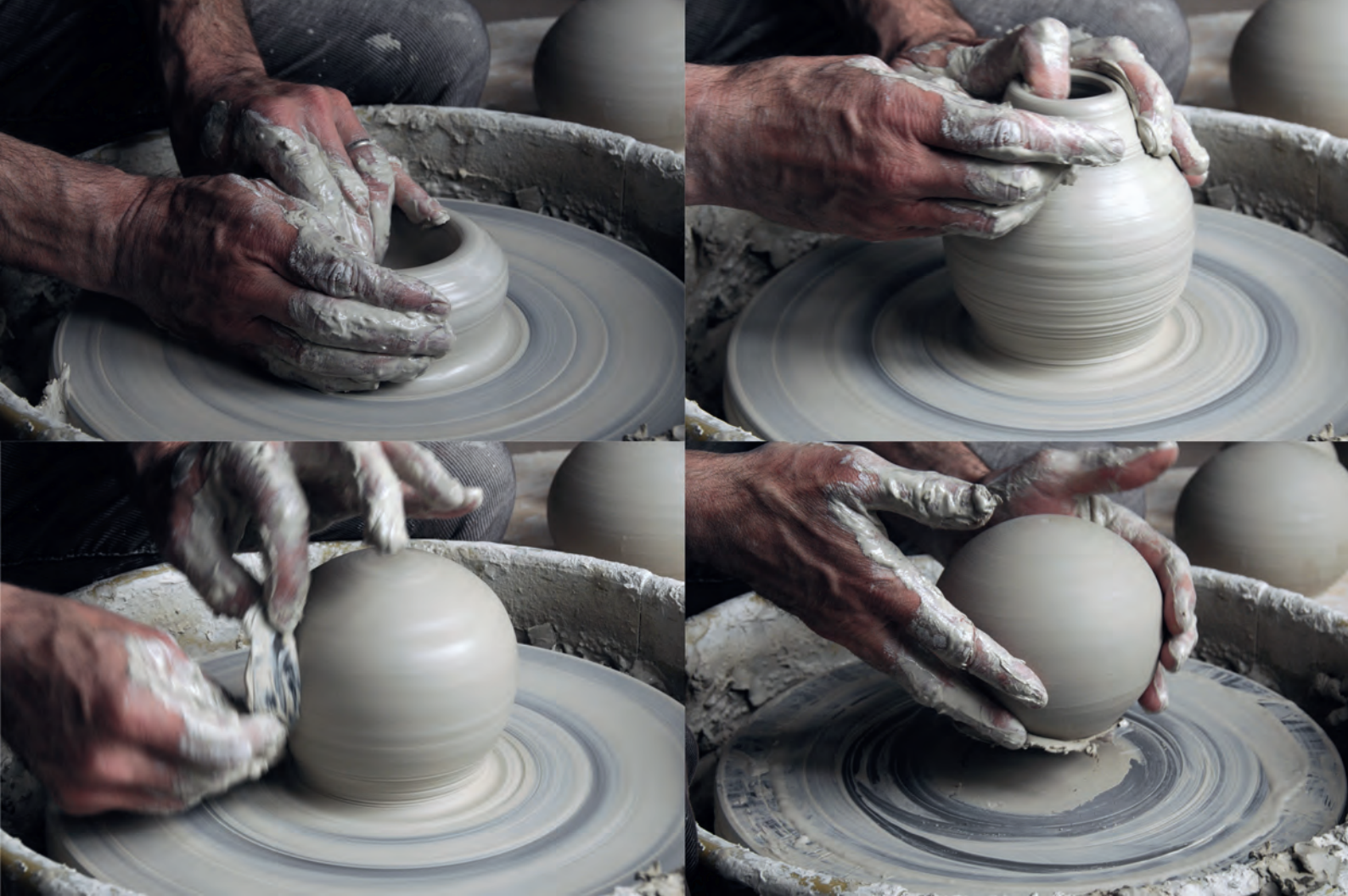
Figure 1: A clay balloon being made, in part with the help of a thin metal sheet. Photographs by Hanna Stahle.
