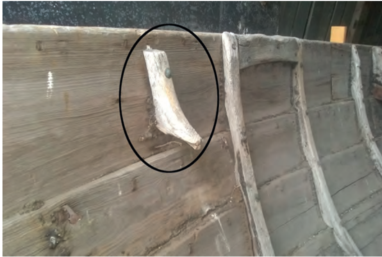
Figure 4: This grown knee can reveal how another part of the boat has been repaired. Photograph by Fredrik Leijonhufvud.
