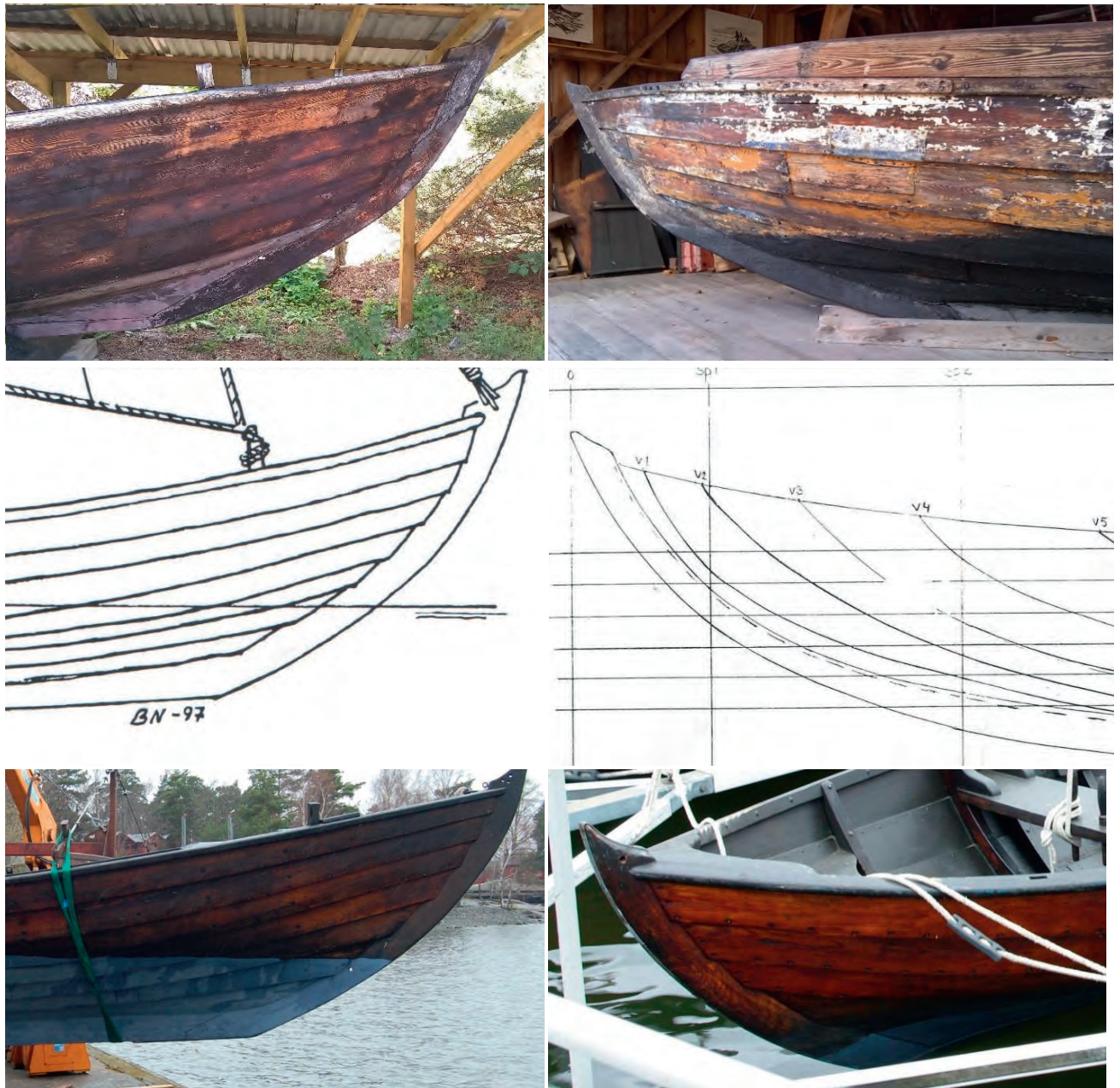
Figure 5 A–F: Two nineteenth-century boats from the Stockholm archipelago, interpreted in reconstructions, but lacking the characteristic shape of the stem. A–B show the original boats, C–D show the line plans from the documentations. E–F show the replicas. Images by Fredrik Leijonhufvud.
