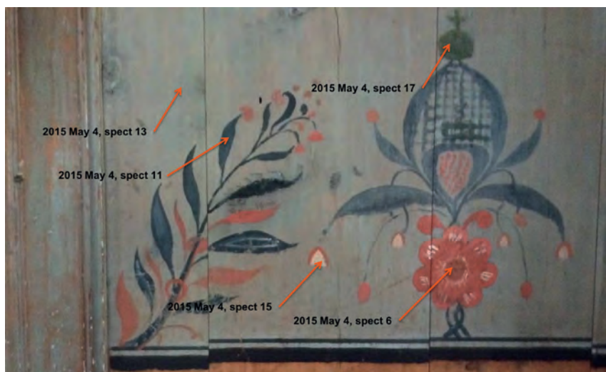
Figure 4: XRF analyses performed on site at Bortom åa Fågelsjö. Photograph by Jacob Thomas.
