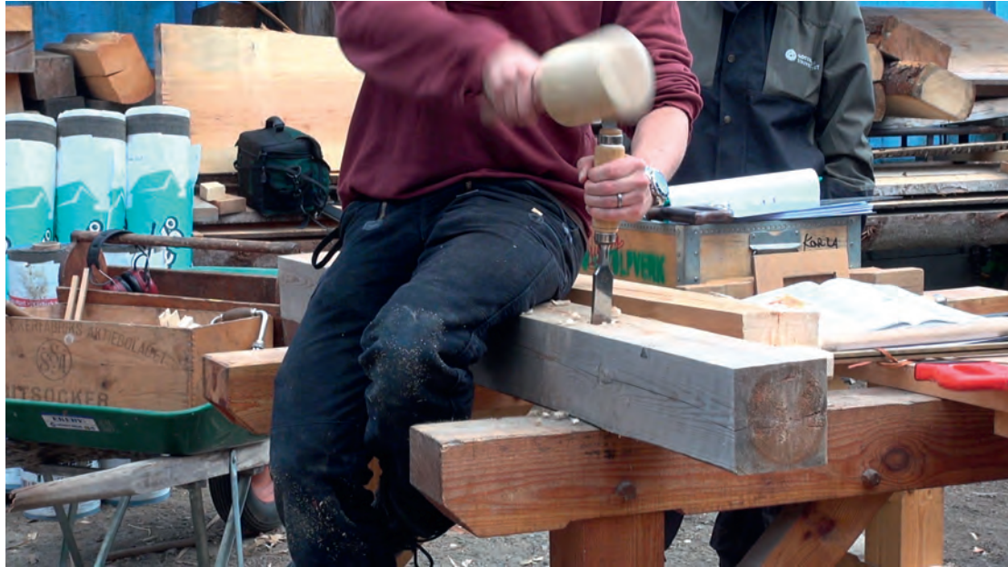
Figure 6: Video sequence of me teaching, demonstrating how I cut a mortice. Click the image to see the video if reading a pdf version, scan the code to the right or go to: https://youtu.be/cBSERnzhn2Y . Video by Ulrik Hjort Lassen.
