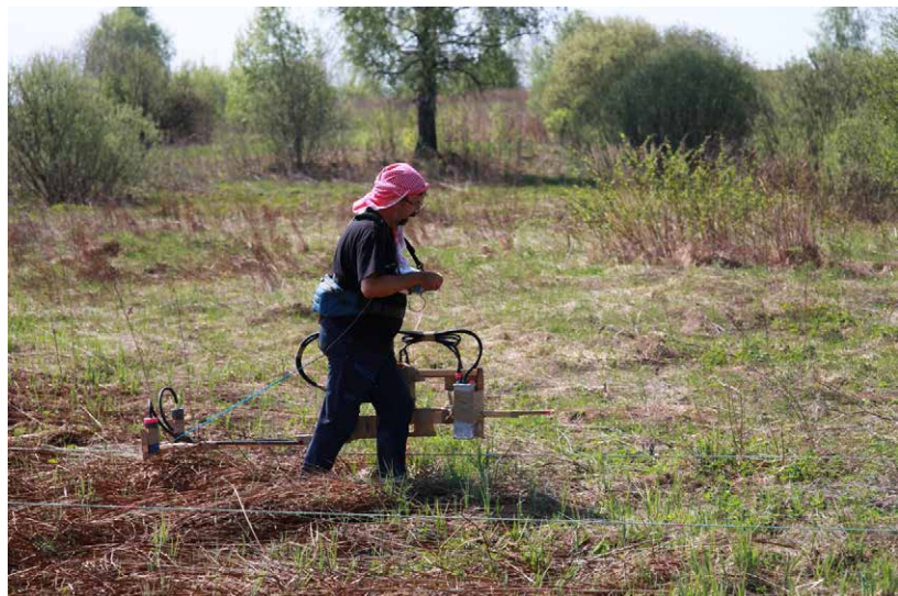
Figure 10: Magnetometer prospecting in action with the handheld duo-sensor cesium magnetometer at Dubokray (Photo: Dima Michaylov).
