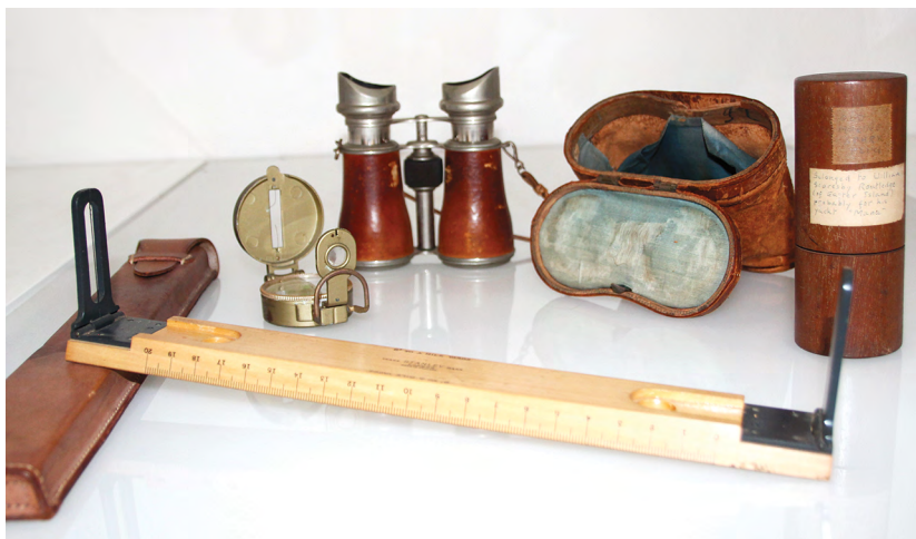
Figure 18.4. Boxwood alidade by Stanley, London with leather case (left); binoculars with leather case lined in blue silk (background); brass directional compass (foreground) and round wood case containing a sparkplug for yacht Mana (right).
