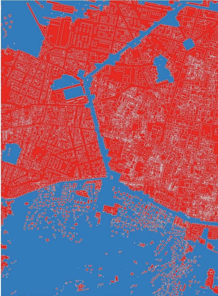
Fig. 10: Uwe Schröder, “Rotblauplan” (red-blue plan) indicating enclosed and open urban spaces, Bologna (der architect 6 (2020))
