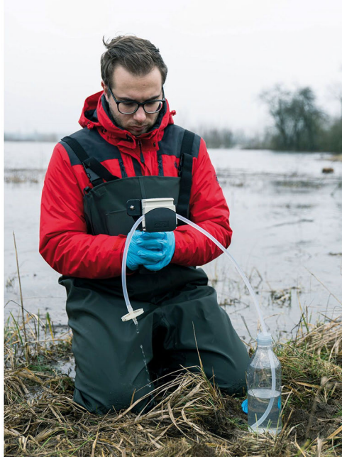
Fig. 4: The collected water is pumped through a special encapsulated filter to isolate the eDNA from the water
