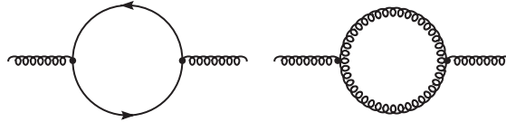
Fig. 2.3 The leading quantum corrections to the running of the QCD coupling constant \alpha_s : gluon self energy at one loop order (ghost diagrams are ignored).
