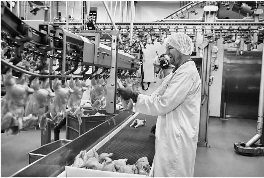
Figure 2.5 Slaughterhouse workers by conveyor belt at Nortura's chicken facility at Hærland, Norway's biggest. Almost completely robotized and automated, the facility at full capacity kills and processes 12,500 chickens an hour, or 3.5 chickens a second.
