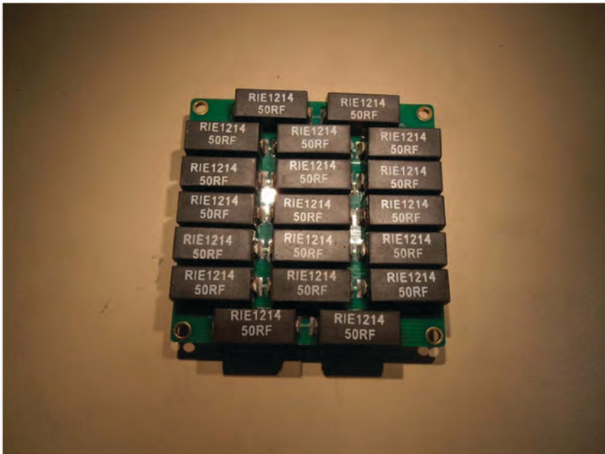
Figure 3.10 Resistors surface mounted onto high temperature printed circuit board.
