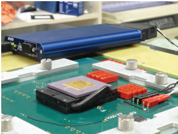
Figure 5.13 HIGHTECS ASIC in PGA package connected to ARINC 429 data reader.
