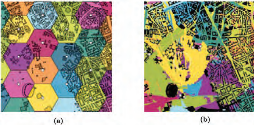
Figure 6.7 Cellular layouts: (a) Idealised hexagonal cells, and (b) Realistic irregular cells.
