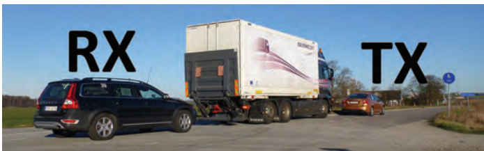
Figure 4.3 The two cars at TX/RX and the truck as obstacle used in the measurements. The total truck length was 980 cm with a container width of 260 cm and height of 400 cm from the ground.
