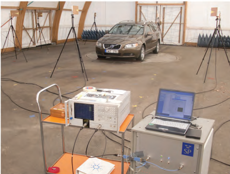
Figure 4.10 (OTA) multi-probe setup for a car at Volvo Cars test facilities [NHA + 14].
