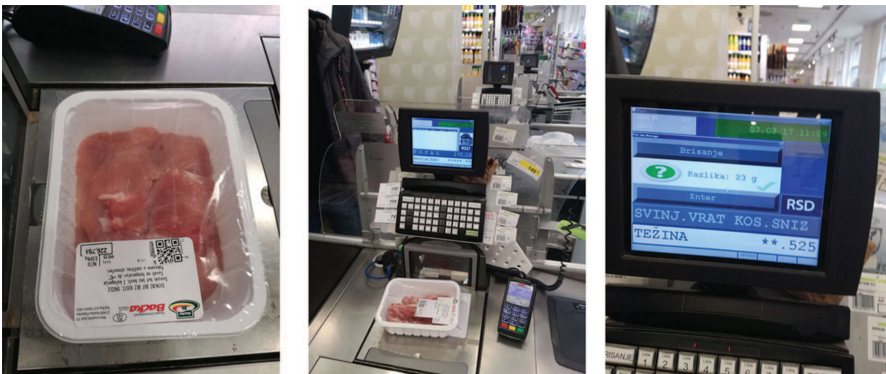
Figure 9.15 Dynamic pricing scenario; different price calculated and displayed based on SmartTag information.
