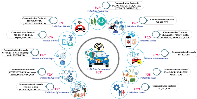
Figure 6.1 Automated vehicle connectivity domains of interaction [1, 13].
