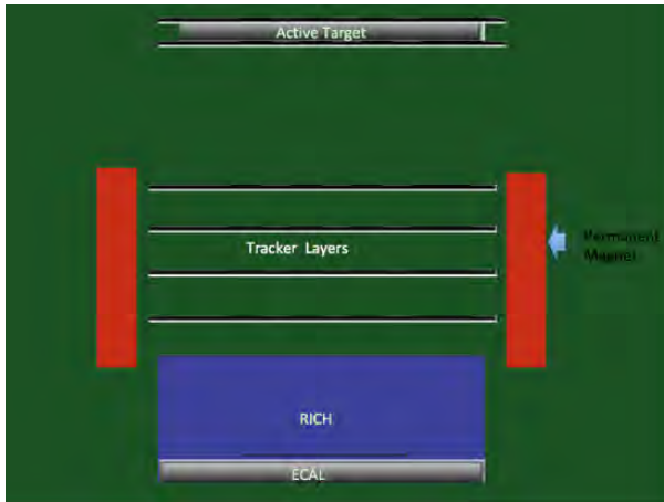
Fig. 5. Structure of the detector proposed as a payload of a satellite dedicate to the measurement of epsilon in a low gravity environment.
