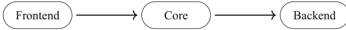
Fig. 3. The design of autoBLAS is divided in three independent components: the user-facing frontend, the optimizing core, and the executing backend.
