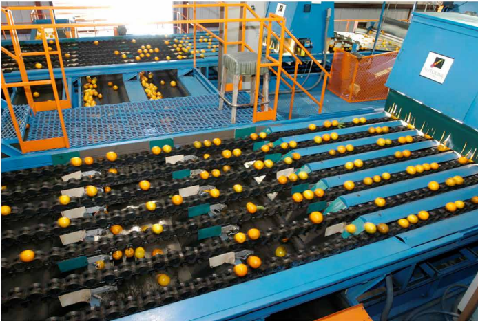
Figure 1 Typical chain involved in production, transport, storage and/or ripening and marketing of fresh produce (top panel) and an image of a grading line - the one point in the chain where all produce items can be inspected individually (bottom panel). (Image source: https://search.creativecommons.org/photos/aaa81a9d-38a4-4b72-9fa5-912b03c61eeb ).
