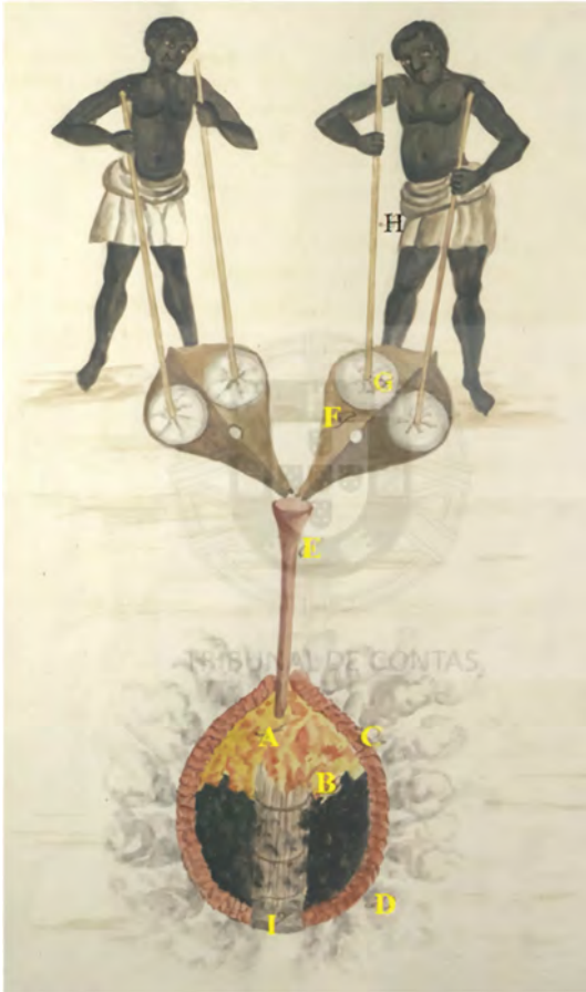
Fig. 3: Iron smelting in Nova Oeiras, 1797. José Álvares Maciel, “Narrative about the Iron Foundry of Nova Oeiras in the Kingdom of Angola,” AHTC, Erário Régio, 4196. Legend: “A – this is a mabú 46 or straw drench, which is placed at the furnace’s center; B – this is the iron covered with charcoal, which is placed on the sides of the same straw, which, in turn, is covered with the same charcoal. The clay tube is used to keep the fire lit and control the temperature; C – this is the furnace’s wall with a tile shard grid. D – this is the smoke exiting the openings of the same wall; E – equally at the reach of the bellows; F – the tube reaches the ore; G – this is the leather of the bellows; H – this is the stick; I – the iron smelted from ore, at the reach of the bellows. This is the smelting of the ore itself, and I placed two arrobas and six pounds of iron ore. In four hours, I saw the smelting of [the number is missing on the manuscript] pounds of iron”.
