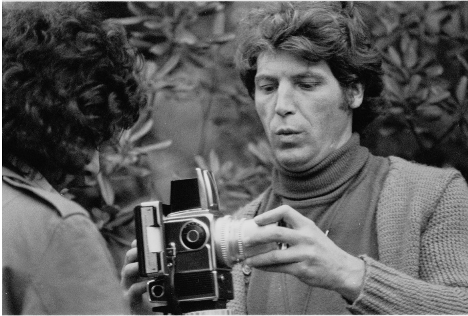
Figure 27: Assistant photographer Pierre Richer, captured while changing the lens of the Hasselblad camera. On the back side of the camera a magazine for Polaroid film is mounted. Private collection Michel Courant.
