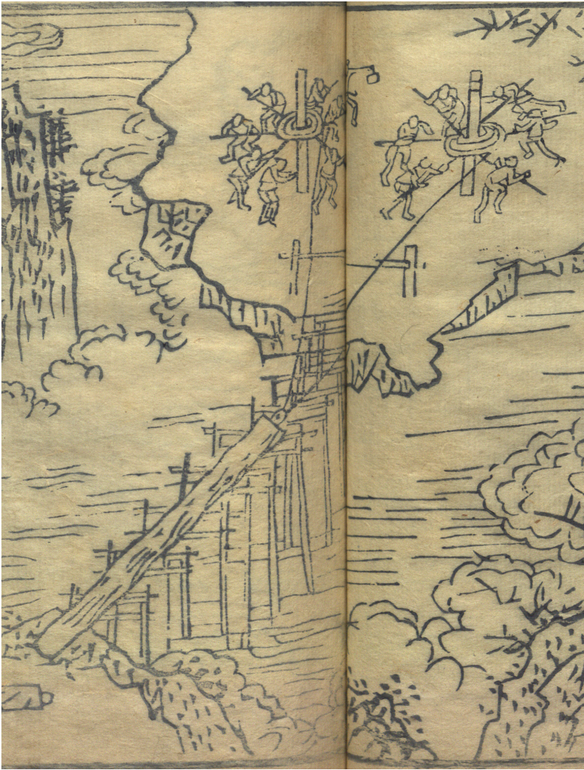
FIG 7.2 Capstan across a chasm. Detail of a woodcut from Essays on Timber Rafting in the Western Regions (Xi cha huicao; 1533). Courtesy of the Library of Congress, Chinese Rare Book Digital Collection.
