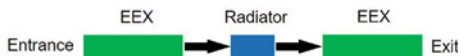
Fig. 3.7 Application of two transverse-longitudinal emittance exchangers to manipulate the bunch length in a storage ring
